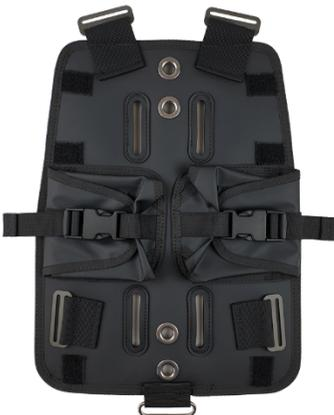
The full-size Formula Soft Backplate is techno polymer layered with TPU coated 420 denier high tenacity nylon front & back. Mesh line backplate soft pad made with 20mm thick open cell foam to minimize water retention easily mounts to the soft backplate using marine engineered hook & loops. 2x 5lb (2.2kg per side) weight pockets are integrated to the soft backplate
